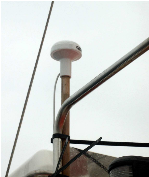
Figure 2-1: The position of the antenna for the Garmin GPS152 unit
